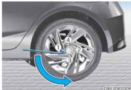
6. Loosen the wheel lug nuts counterclockwise one turn each in the order shown above, but do not remove any lug nuts until the tire has been raised off of the ground.
