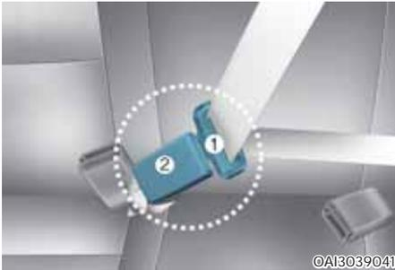
Insert the tongue plate (1) into the buckle (2) until an audible “click” is heard, indicating the latch is locked. Make sure the belt is not twisted. When using the rear center seat belt, the buckle with the “CENTER” mark must be used.
