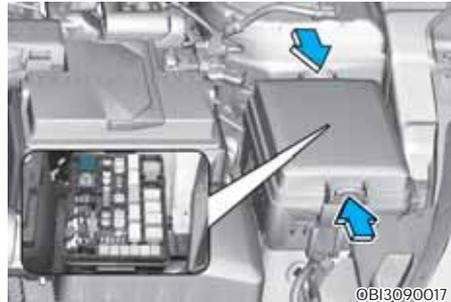
If the multi fuse is blown, it must be removed as follows:
