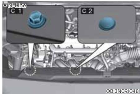
2. Remove retainers available on under cover bottom area in the respective side of headlight for bulb A/S.
