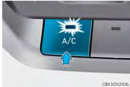
Push the A/C button to manually turn the system on (indicator light will illuminate) and off.
