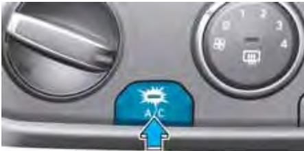
Press the A/C button to turn the air conditioning system on (indicator light will illuminate). Press the button again to turn the air conditioning system off.
