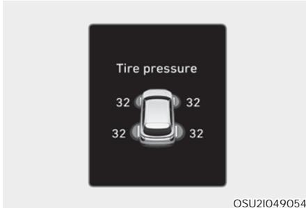
When the tire pressure monitoring system warning indicators are illuminated and a warning message displayed on the cluster LCD display, one or more of your tires is significantly under-inflated. The low tire pressure position telltale light will indicate which tire is significantly under-inflated by illuminating the corresponding position light.
