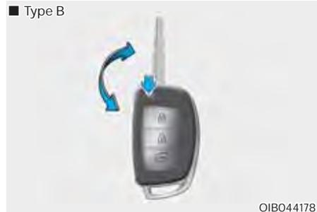
If the remote key does not operate normally, you can lock or unlock the door by using the mechanical key.
