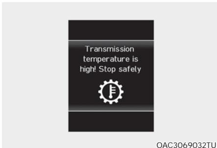
The following extreme cases may damage the clutch due to overheating while driving. Vehicle's own protection system sounds alarm and displays warning messages. Please shift into lower gear or stop the vehicle according to the instruction.
