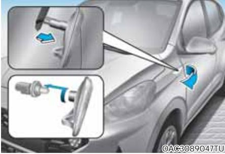
1. Remove the lamp assembly from the vehicle by prying the lens and pulling the assembly out.
