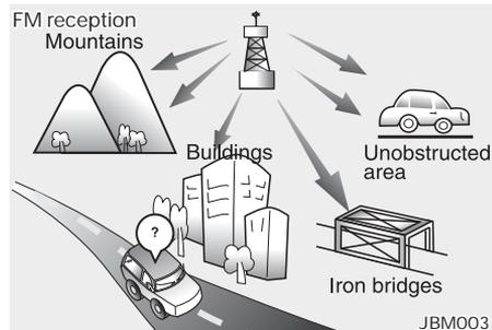
FM broadcasts are transmitted at high frequencies and do not bend to follow the earth's surface. Because of this, FM broadcasts generally begin to fade within short distances from the station. Also, FM signals are easily affected by buildings, mountains, and obstructions. This can lead to undesirable or unpleasant listening conditions which might lead you to believe a problem exists with your radio.
