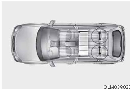
ISOFIX anchorages have been provided in the left and right outboard rear seating positions. Their locations are shown in the illustration. There are no ISOFIX anchorages provided for the center rear seating position.
