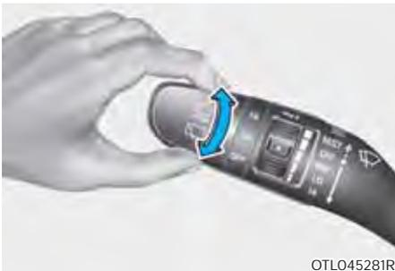
The rear window wiper and washer switches are located at the end of the wiper and washer switch lever.
