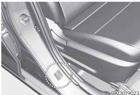
The tires supplied on your new vehicle are chosen to provide the best performance for normal driving. The tire label located on the driver's side center pillar gives the tire pressures recommended for your car.
