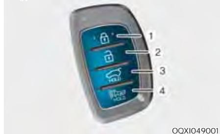
Your HYUNDAI uses a Smart Key, which you can use to lock or unlock a door (and tailgate) and even start the engine.
