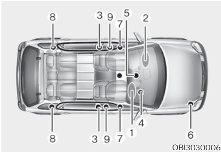
The SRS consists of the following components:
