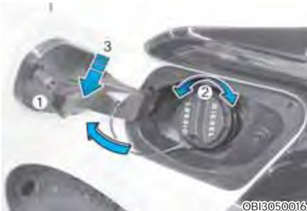
3. Pull the fuel filler door out (1) to fully open.
