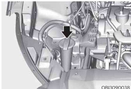
Check the fluid level in the washer fluid reservoir and add fluid if necessary. Plain water may be used if washer fluid is not available.
