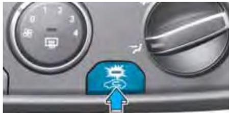
This button is used to select the outside (fresh) air position or recirculated air position.
