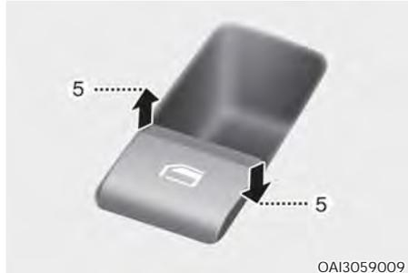
To open or close a window, press down or pull up the front portion of the corresponding switch to the first detent position (5).
