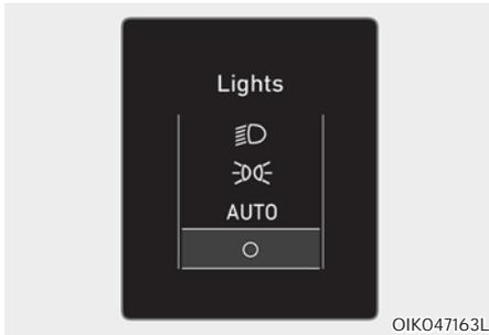
This indicator displays which exterior light is selected using the lighting control.
