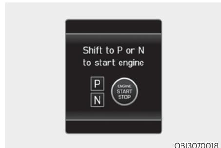
Vehicle with dual clutch transmission/
