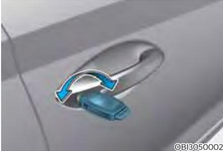
Turn the key toward the rear of the vehicle to unlock and toward the front of the vehicle to lock.
