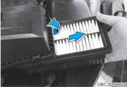
1. Loosen the air cleaner cover attaching clips and open the cover.
