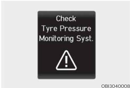
This warning message is displayed if the tire pressure is low. The corresponding tire on the vehicle will be illuminated.
