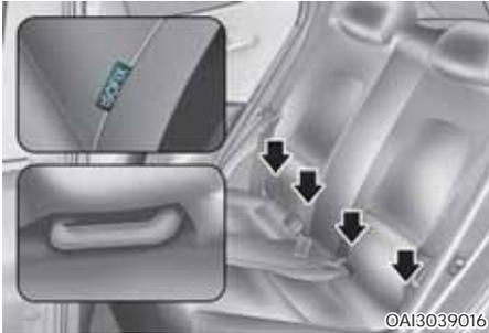
The ISOFIX anchorage symbols are located on the left and right rear seat cushions to identify the position of the ISOFIX anchorages in your vehicle (see arrows in illustration).
