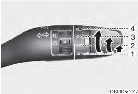
To operate the lights, turn the knob at the end of the control lever to one of the following positions:
