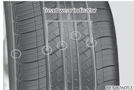
If the tire is worn evenly, a tread wear indicator will appear as a solid band across the tread. This shows there is less than 1.6 mm (1/16 inch) of tread left on the tire. Replace the tire when this happens.
