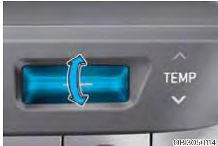
The temperature will increase by pushing the switch to up.
