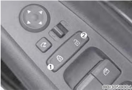
When pressing the (🔒) portion (1) of the switch, all vehicle doors will lock.
