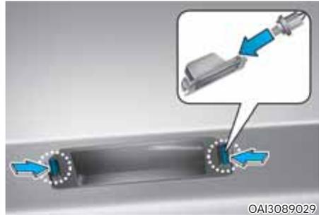
1. Using a flat-blade screwdriver gently pry the lens cover from the lamp housing.
