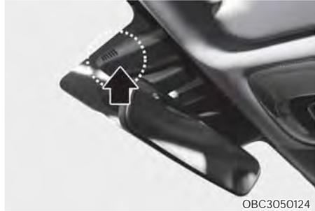
Auto defogging helps reduce the possibility of fogging up the inside of the windshield by automatically sensing the moisture on inside the windshield.
