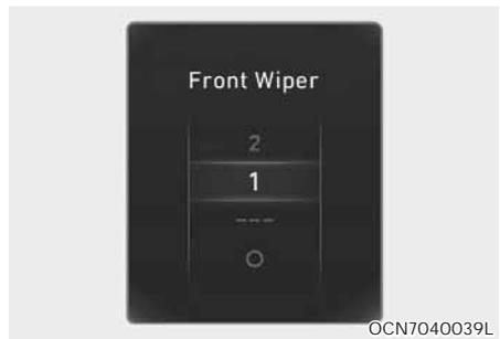
This indicator displays which wiper speed is selected using the wiper control.
