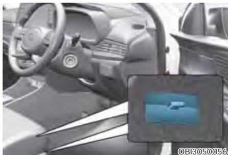
ALWAYS use the Floor Mat Anchors to attach the front floor mats to the vehicle. The anchors on the front floor carpet keep the floor mats from sliding forward.
