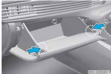
2. Push in both sides of the glove box as shown. This will ensure that the glove box stopper pins will get released from its holding location allowing the glove box to hang.
