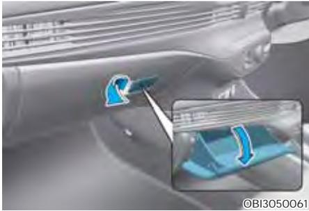
To open the glove box, pull the lever and the glove box will automatically open. Close the glove box after use.
