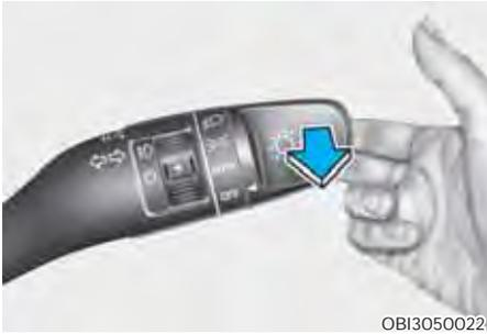
To flash the high beam headlights, pull the lever towards you, then release the lever. The high beams will remain ON as long as you hold the lever towards you.
