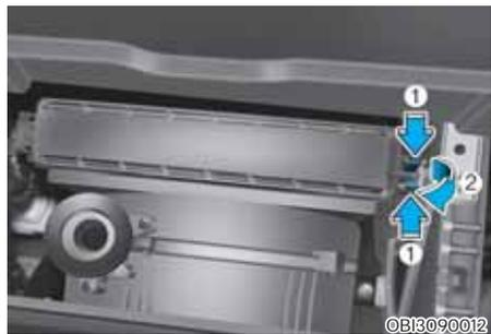
3. Remove the climate control air filter cover by pushing or pressing the clip (1) on right side.
