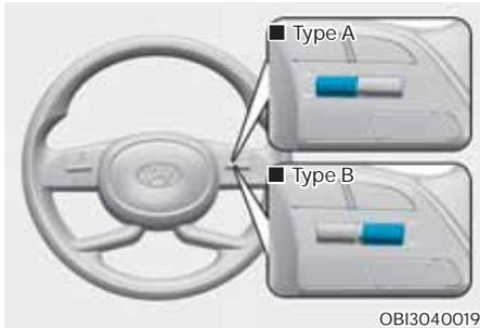
To change the trip mode, toggle the “^, v” switch on the steering wheel.
