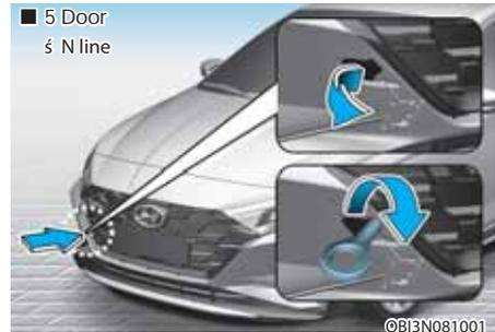
1. Open the tailgate/trunk, and remove the towing hook from the tool case.
