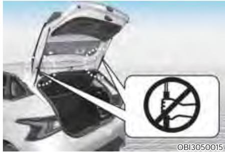
Do not hold the part (gas lifter) that supports the tailgate. Be aware that the deformation of the part may cause vehicle damage and a risk of safety accident.
