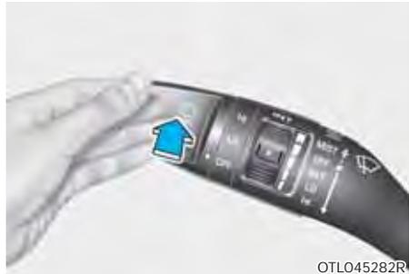
Push the lever away from you to spray rear washer fluid and to run the rear wipers 1-3 cycles. The spray and wiper operation will continue until you release the lever (if equipped).
