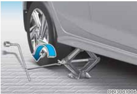
8. Insert the jack handle into the jack and turn it clockwise, raising the vehicle until the tire clears the ground. Before removing the wheel lug nuts, make sure the vehicle is stable on the jack.
