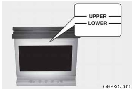
**If your vehicle is equipped with a battery marked with LOWER (MIN) and UPPER (MAX) on the side, you should check the electrolyte level.**
