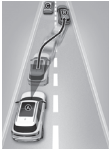
[A] Your vehicle [B] Lane changing vehicle [C] Same lane vehicle or powered two-wheeler
