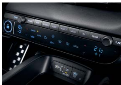
Dual-zone full automatic air conditioning (with micro air filter, auto defog system, fine dust sensor, air cleaning mode, and after-blow function)
