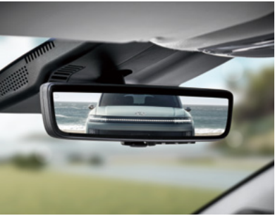
Compact Digital Side Mirror Digital Center Mirror with Camera Cleaning System
