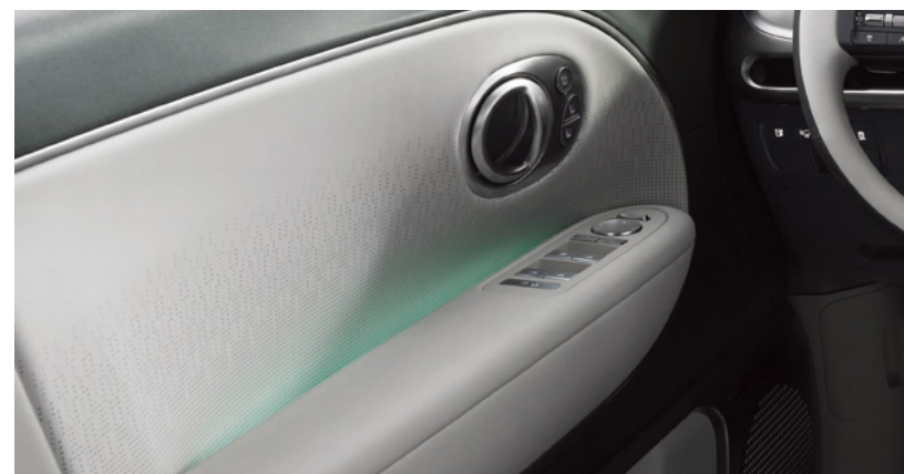
Synthetic leather(door center trim with digital design punching)
