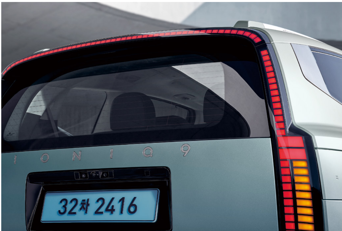
Rear Led Combination Lamps, Led Supplemental Brake Lights
