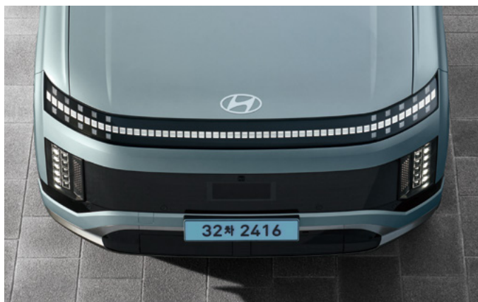
Small-Cube Projection Led Headlamps (Daytime Lights, Positioning Lamps, Turn Signals)
