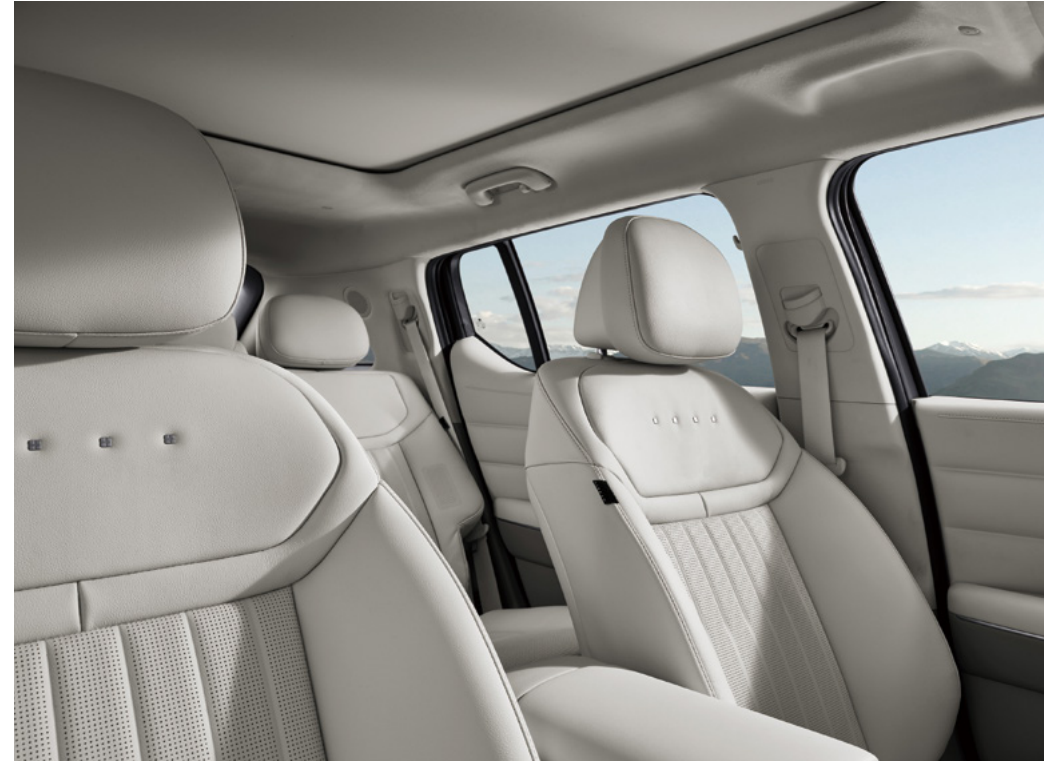
Bio-processed natural leather seats(metal patch applied, embossed design punching), Recycled PET suede interior materials(headlining/sun visor)
